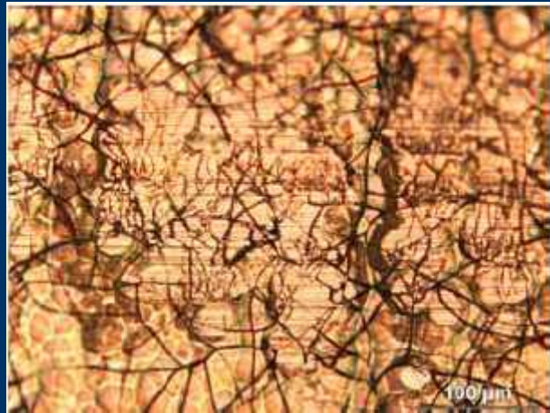
Fretting test track 5,000 cycles Al 2 O 3
