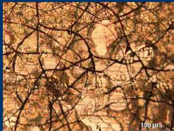
Fretting test track – 5,000 cycles
